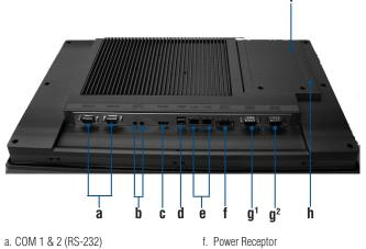
a. CUM 1 & 2 (RS-232) b. Audio (Line out, Mic in) c. HDMI d. USB 2.0 e. LAN (10/100/1000) f. Power Receptor g<sup>1</sup>.COM3 (RS-232) g<sup>2</sup>.COM4 (RS-422/485) h. Mini PCI-E slot i. 2.5" SATA HDD Housing
