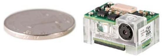
*With its compact dimensions and integrated decoder, the N3680 2D imager makes it easy to incorporate high-performance scanning into your designs.*
